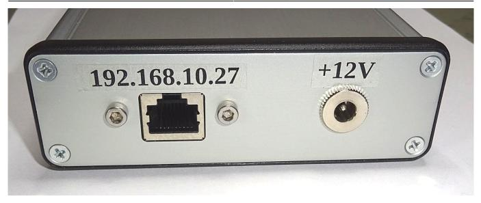
Before assembling the case you have to configure the IP address, because this is only possible via USB. At the same time I installed the F50EO firmware to make the Pluto usable for DATV,
