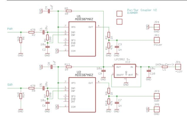
the 1.8kOhm resistor is in parallel with the 56 Ohm resistor (schematic above), together with R8 and the input resistor of the AD8307 you get 50 Ohm.
