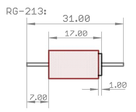
On the left, the cable is cut flush to the inner conductor. On the right side 1mm of the shield is left, here the ground is connected.
