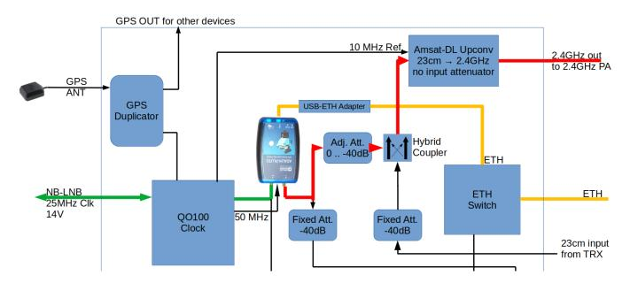
The SDR software accesses the NB-Pluto via Ethernet. This is connected with a USB/ETH adapter and has a fixed IP address.
