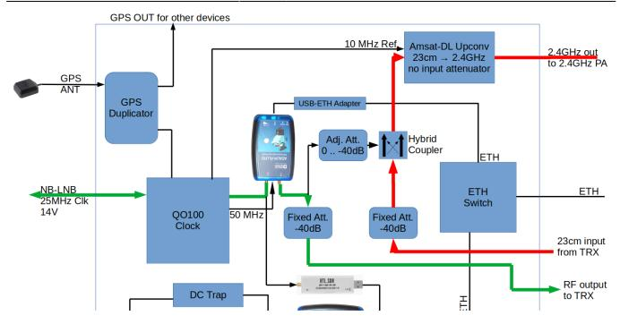
The receive signal (green) comes from the LNB and goes through the clock board where 13.8V supply is fed as well as the 25 MHz LNB clock. Finally, the receive signal is fed to the RX input of the Pluto. This is the same as before in SDR mode.
