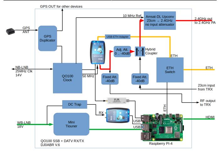
The receive signal (green) goes from the LNB to the minitiouner, which also generates the 18V supply for the LNB.
