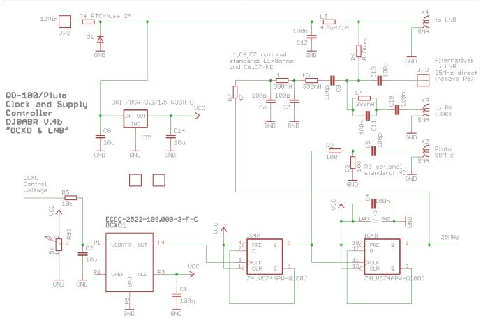
On the board (which fits into a common 74x55mm tinplate case) is an SMA connector for connecting the sat cable. This is connected to an SMA socket for the receiver. The LNB supply is fed via a 4.7uH choke (phantom power). At a voltage of 13.8 or 12V the LNB switches to polarization for the NB transponder of QO-100.
