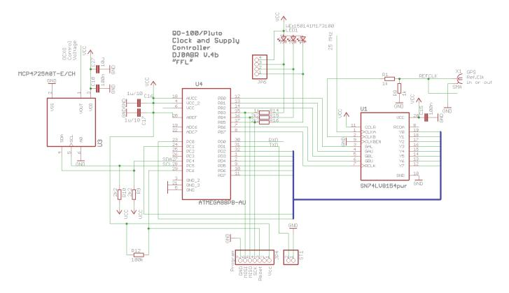
A 16 bit counter is used to count both the 25 MHz LNB clock and the 10 MHz reference signal. By comparing both signals by software, the actual frequency of the 25 MHz signal is measured, with an accuracy of 0.01Hz. From the deviation a correction value is formed, which fine tunes the OCXO via a 12bit DAC as control voltage.
