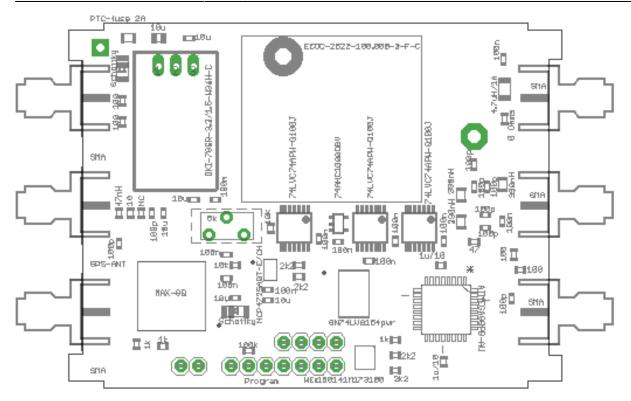
the PCB is designed for a tinplate case 72x55mm.
