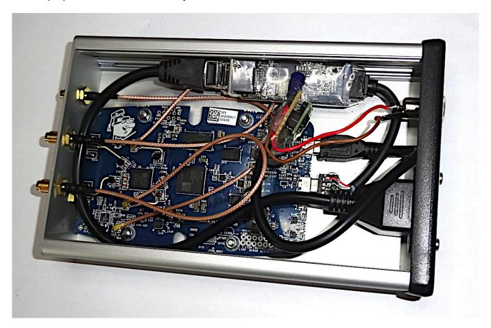
Clock and RX/TX2 are available on U.Fl connectors. Suitable SMA adapters are available at e.g. ebay.
