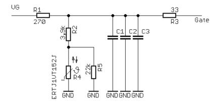
after longer tests with higher temperatures it turned out that the quiescent current does increase slightly with temperature, so the resistor R2 was reduced to 3.3k.
