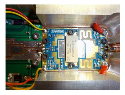
Detailed view of the PA. Note the 2.4 GHz input and output connectors. Here you really have to work RF-optimally. The connections must be as short as possible. At the output, a "hood" of solder wire was placed around the semi-rigid cable to get a reasonable match as far as possible. At power levels up to 250 watts, any attenuation acts like a heater and can cause damage.
