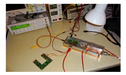
the PA in test mode. The board in front generates the gate bias for the 250W module. This board was designed and built by DG8FAC and is also in the QO-100 station at the Antarctic station. It is a 5V voltage regulator, an analog switch and a potentiometer for quiescent current adjustment. To achieve the desired gain of +17dB in linear mode, a quiescent current of about 800mA must be set.
