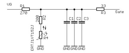
our bias voltage of approx. 1.8 volts is present at the VG connection. When the module temperature rises, R4 becomes less resistive and pulls down the voltage. So the effect of R4 has to be reduced.
