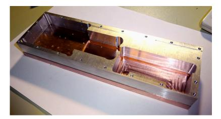
before the boards are mounted, the side holes for all connectors have to be milled.
