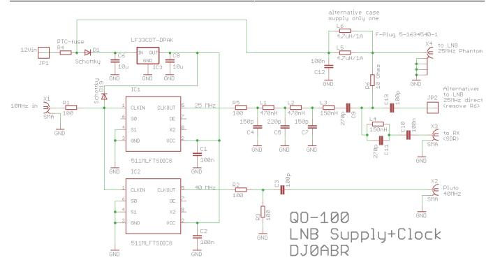
The usual station power supply of 13.8 (12) volts is applied to the satellite cable via a choke (phantom power). This supplies the LNB and also sets the correct polarity.
