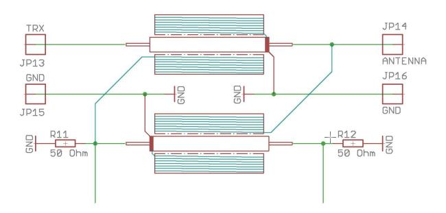
the upper toroid measures the current through the inner conductor of the antenna cable and the lower toroid measures the voltage at the antenna connector. Together with the 50 ohm resistors, this measuring bridge produces an RF signal corresponding to the forward power and one corresponding to the return power.
