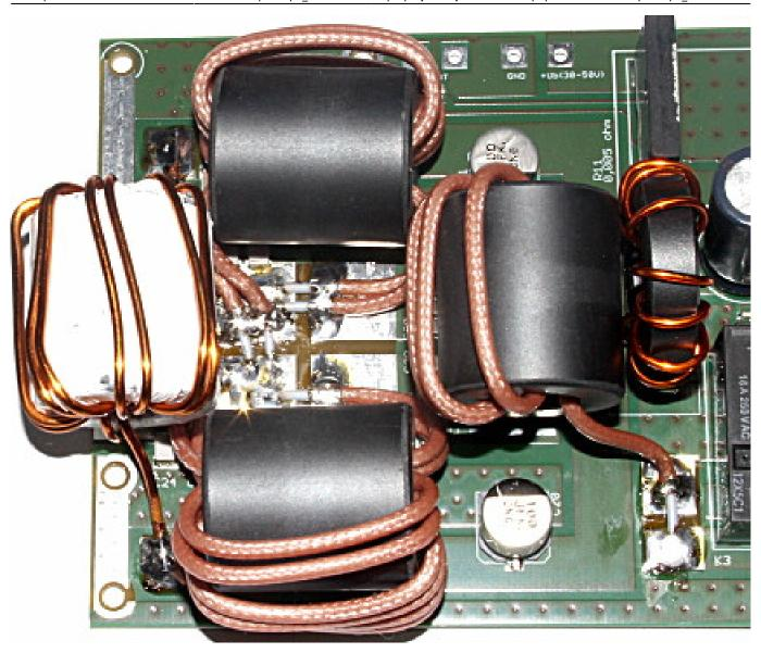
The white choke on the left is for the power supply, and to the right is TR3 and TR4. These two tube cores are responsible for the impedance transformation. On the right there is another balun to create an unbalanced output signal.
