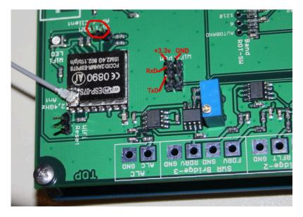
This connector has a ground and 3.3v pin to supply the level converter (if required). Some level converters use the PC's USB port for supply, in this case, you need to connect only the ground pin.
