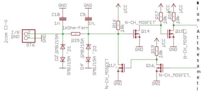
me the input is HF-filtered with two 1nF Cs and one ferrite. Since a possible overvoltage pulse behind the ferrite is already significantly reduced, two more TVS diodes follow here, which dissipate the rest. I equipped two of the connections like this. The CIV connections, which are connected to transceivers over a short distance, do not have TVS diodes.
