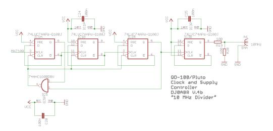
10 MHz is generated from the 100 MHz OCXO. This frequency can be used for a transceiver (e.g. IC9700) or also frequency counters, etc.
