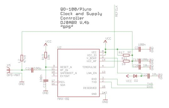
an Ublox MAX-8Q is used. This module is inexpensive and has a programmable reference output (10 MHz).
